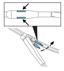
3. Attach the new blade to the arm and snap it into place.
